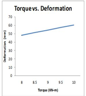
Fig. 3.6 (a) Torque Vs Maximum Deformation of Ladder Chassis
