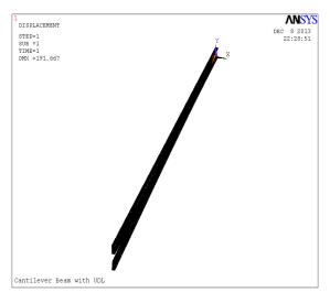
Fig. 2.2 (a) Deformation of cantilever beam
