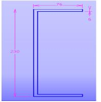
Fig. 2.1 (a) C- section of side member
