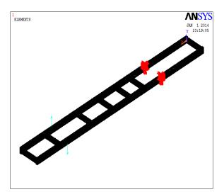
Fig. 3.6 boundary condition and load condition on ladder frame chassis
