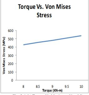
Fig. 3.6 (b) Torque Vs Maximum Von Mises Stress of Ladder Chassis
