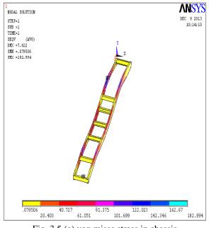
Fig. 3.5 (a) von mises stress in chassis
